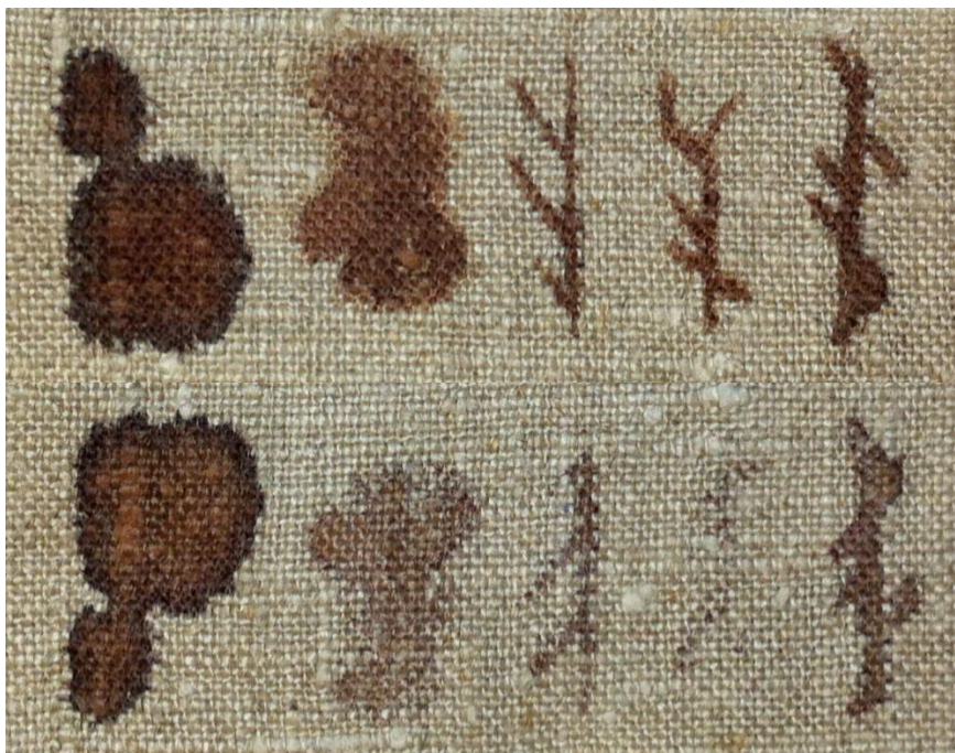
Figure 10. Forward (top) side and reverse side of German linen painted with pig blood that was stirred to prevent coagulation. Notice reddish tint of blood and the dark perimeter.
