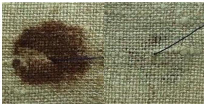
Figure 18. Blood transfer from aloe-covered leather whose surface contained clotted dry blood. Forward side and the mirror image of reverse side are shown. A blue thread was passed through the linen to help correlate forward and reverse sides. Only a tiny reverse image is present.
