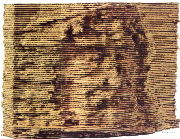
Figure 18: Three dimensional model made by cutting out microdensitometer data graphs on cardboard and assembling them.
