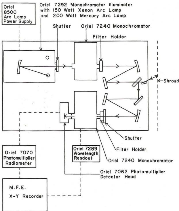
Fig. 3. Oriel reflectometer/fluorimeter schematic layout.
