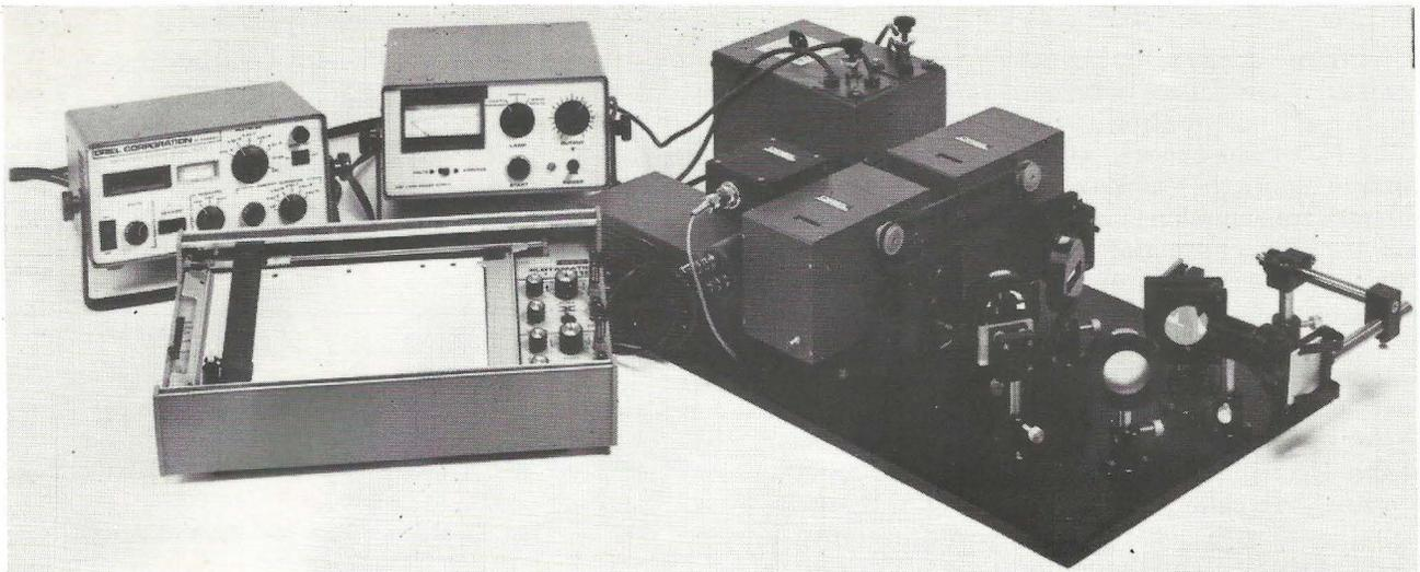
Fig. 2. Oriel reflectometer/fluorimeter with cover removed with lamp power supply, photomultiplier radiometer, and x-y recorder.
